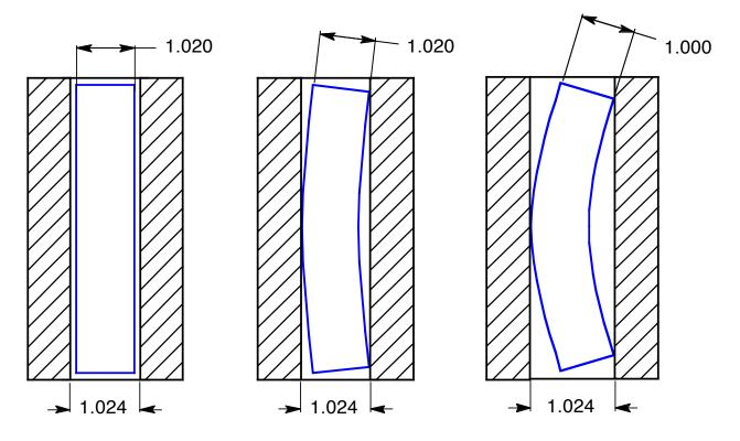
**Figure 5-4** Verification of flatness of a feature of size at MMC with a gage.
