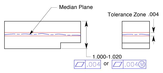
**Figure 5-3** The flatness tolerance of a median plane is associated with the size dimension.
